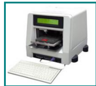
Figure 27. VetScribe™ automatic rabies tag engraver.
